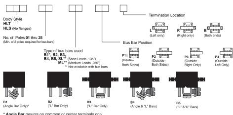
\* Angle Bar mounts on common or center terminals only. †Minimum of 4 Poles Required.
